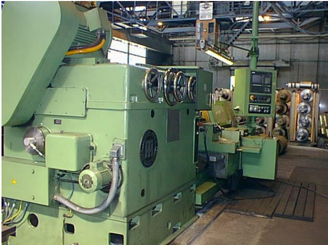
Figure 9: Extremely robust and stable is the headstock. The new spindle motor was put back on the headstock and electrically designed for stepless speed regulation.
