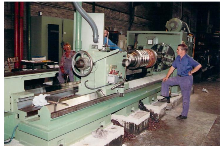
Figure 2: The sub base is being filled with cement, so that the vibrations are damped and that with special cement, which behave properly when dehydration.
