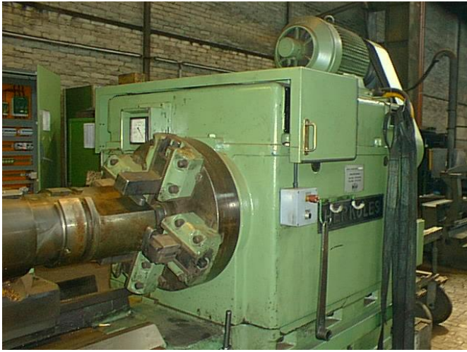
Figure 8: The claws box has the WIAP all revised so that the machine almost like a can work new machine. Often even better than a new one, because today a lot is no longer built as sturdy and stable, as in the old machines.
