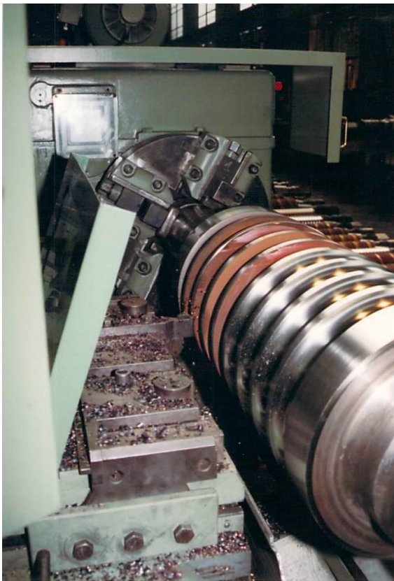
Figure 4: Normal 4 steels were engaged simultaneously. Program test was only one in use.
