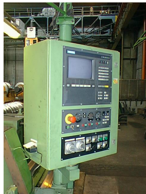
Figure 3: The CNC Sinumerik was equipped with a special program. The WIAP developed parameterized special programs, so that the operators, some of which were about to board, without expertise, respectively. very easily could operate this machine after reconstruction CNC experience.
