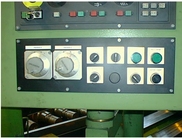
Figure 3: The two axes X and Z have a hand wheel for better scratching at the tool zeroed.
