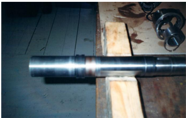
Figure 11: The drive shaft was removed from the headstock. Usually you do everything without a hammer, but with thoughtful deduction solutions.
