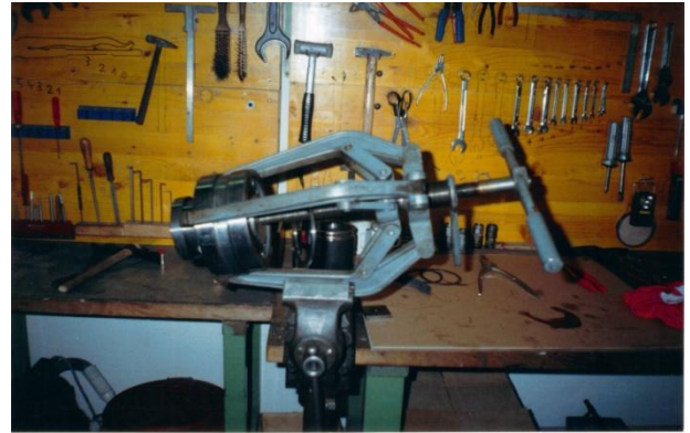
Figure 8: It needs some pullers to pull the gears and bearings.
