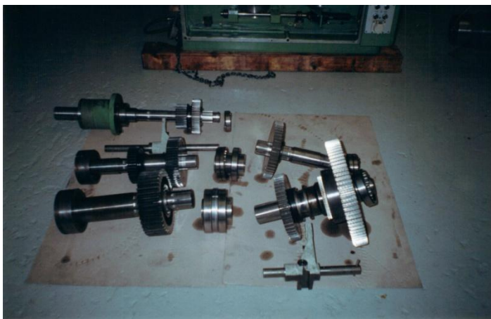
Figure 12: Here everything is laid on the headstock so, so that all spacer rings come back to the right place.
