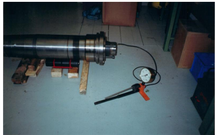
Figure 10: Here is pressed with the Press Association pump the camp. The procedure was very popular a few years. However, when such a pump is missing, which will cost about 3000 CHF and the oil, then the removal can not take place.
