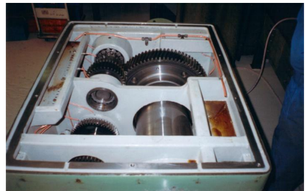
Figure 3: Good construction. From the top of the lid is removable. The headstock damage was bearing damage. He must be opened. For this purpose the headstock was taken in our workshop.
