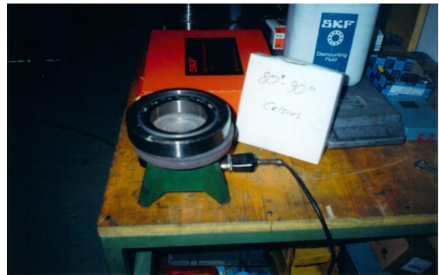
Figure 9: raise spindle bearings again goes well with heat. A hot plate can ease much. It is important to work very clean so that no dirt can get into the camp. Back is also the oil tank for the Press Association Abpressvorrichtung.
