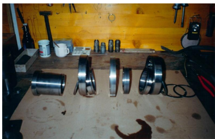
Figure 15: Converted bearings are not replaced, must be handled with great care. Make sure that the cages are not damaged. Always see on which side of the large opening is so is not pressed by
