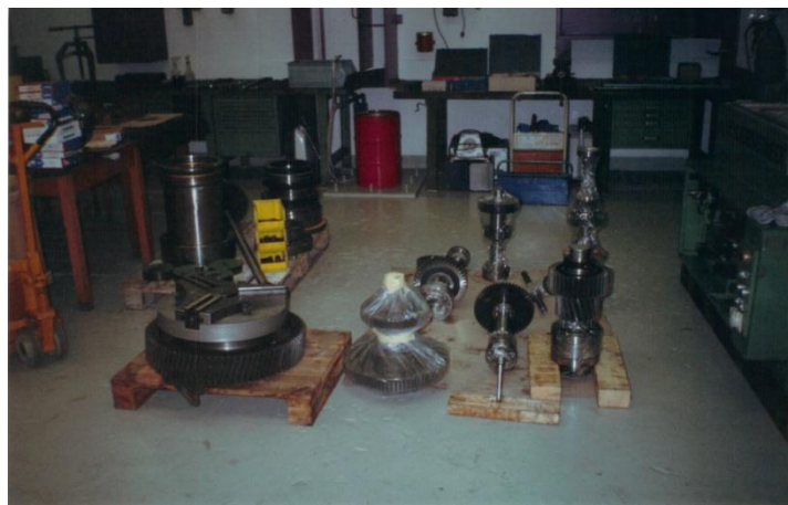
Figure 13: gears, shafts, bushings and bearings are protected with wooden Before blows and impressions.
