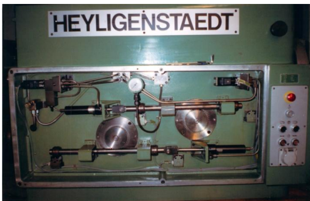
Figure 1: The shift linkage of the shift forks is controlled by cylinder. A thoughtful, intelligent switching solution.
