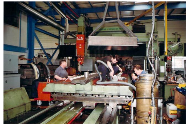
Figure 8: A large machine with a cunningly devised management solution. When planing the stick-slip phenomenon does not interfere. But when milling with a slow feed, it is disturbing.
