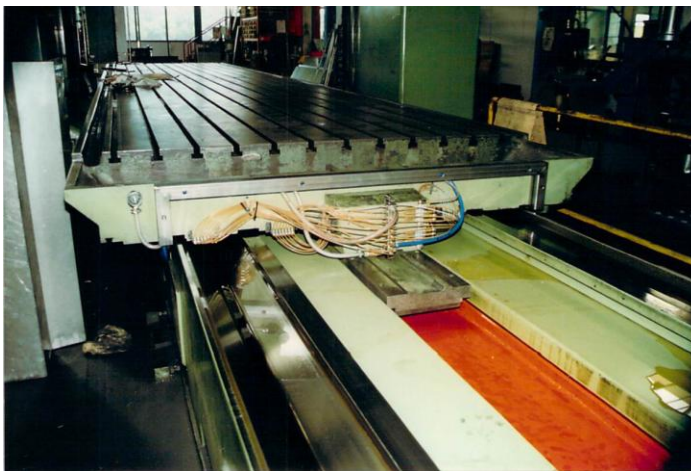
Figure 5: the end face from the 2-part slide the distribution center of the air withdrawal is mounted.
