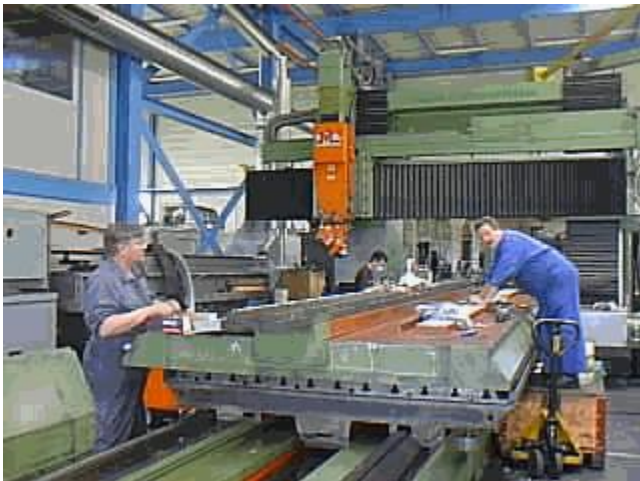
Figure 1: Lubrication at Waldrich planer with air support. Machine made jerks during milling and the so-called Stip Slik effect had to be removed.
