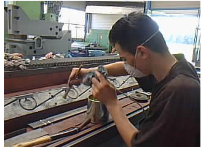
Figure 2: The SKC covering is re-poured. The WIAP apprentice Burim when cleaning the adhesive Ausgiessarbeit.
