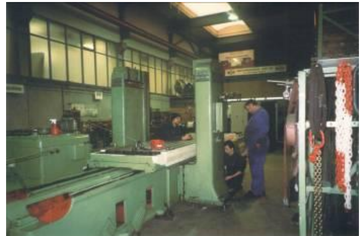
Figure 1: The planer with the shortened side columns. First, we can drill 4 40 H7 pin holes on a boring mill at 0.01 mm accuracy.
