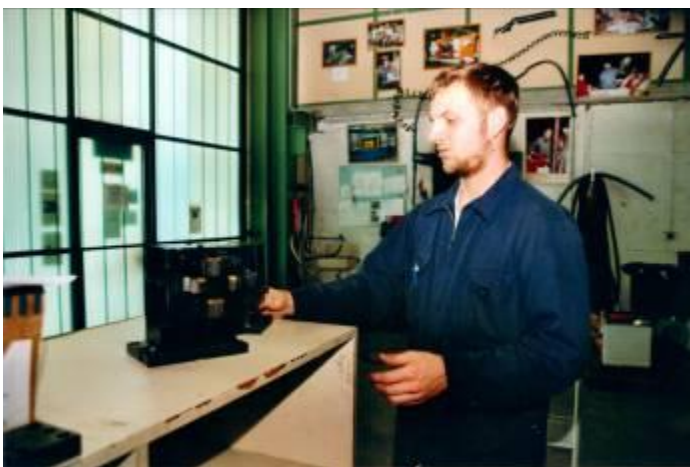
Figure 19: The tool presetting and control whether the preparation is ok according to the drawing.
