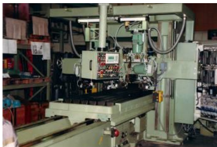
Figure 6: The CNC controller was chosen by a German manufacturer. There have been chosen three modes. Manual, semi-automatic and CNC operation.
