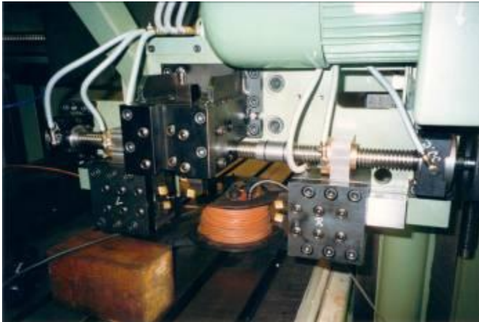
Figure 8: This new slide system was constructed by the WIAP AG so that may be several steels engaged simultaneously.
