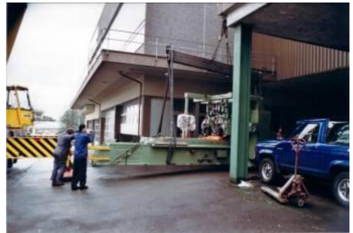
Figure 39: At the retail level the machine with the WIAP Transportjoch could be unloaded.
