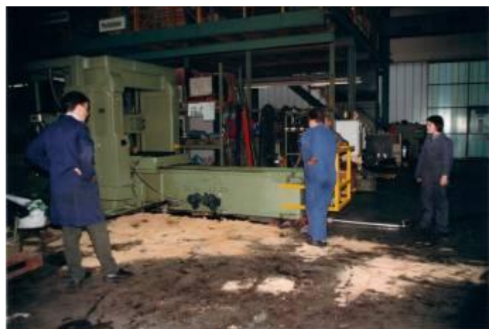
Figure 7: The table drive running with a hydraulic drive, which can be quickly to 70 meters per minute. Since it was a bit oily.
