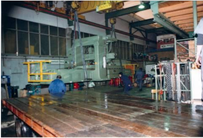
Figure 31: The machine is loaded onto a low-goers trailer.
