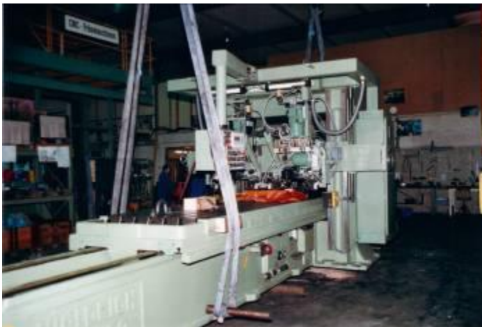
Figure 28: The holes in the bed were at the lower limit for the lifting of the machine. But it had to
