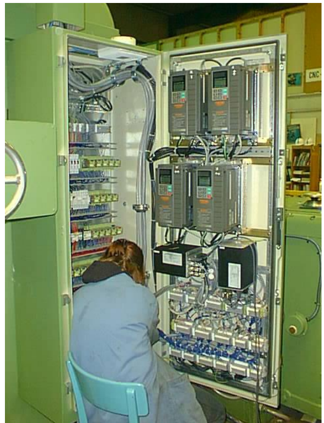
Figure 25: Electrical cabinet assembly of Waldrich planer. Cabinet mounted directly on the machine.
