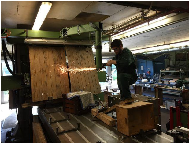
Figure 10: Here, the CNC holding tube had to be shortened slightly so that the workpiece can pass under the control. Good coverage is important that nothing is damaged.
