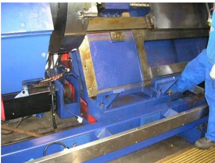
Figure 5: Here was a spacer plate mounted, which had to be dismantled for the larger headstock.
