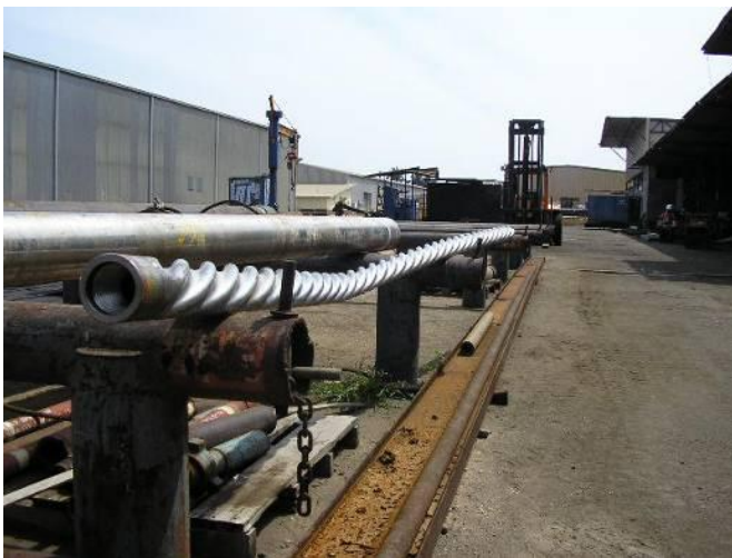
Figure 1: This workpiece was clamped on the fly in the CNC turning machine, the back of the lining about 4 feet to rotate freely. Only under special circumstances was finally told me, how the accident actually happened. Then broken a blast machine.
