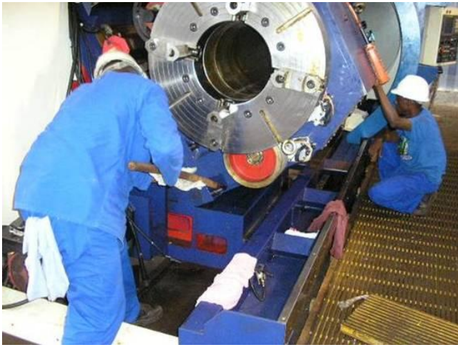
Figure 4: The new spindle stock is ordered with a larger bore. The conventional hole was 250 mm; the new 320 mm.
