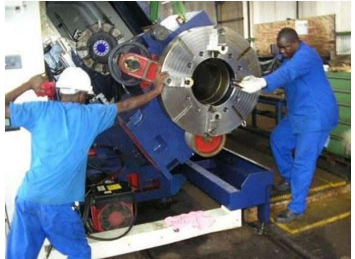
Figure 7: placing a headstock newly Without right crane was not easy.
