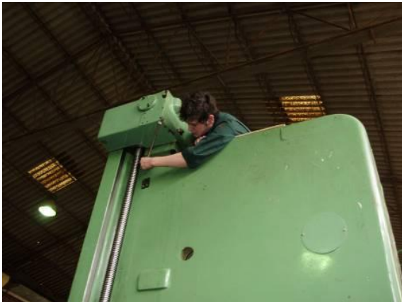
Figure 21: Sven Widmer when tightening the crossbar drive, after the pins have been set, we received from Switzerland, because many middle bolts were no longer available to the machine.
