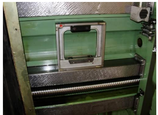
Figure 47: The transom is also checked. If that's not good, it can be set up on the shaft. But since you have to first make a plan rotation.
