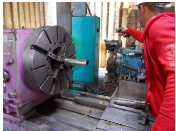
Figure 15: The conicity of the workpiece headstock is determined. 7 pages of minutes for VAM. 14 pages has the internal protocol.
