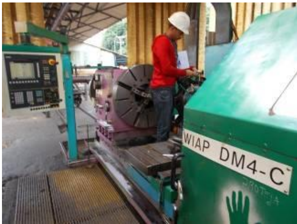
Figure 17: Always the end of June to be replaced on all CNC lathes documents. The geometry test renewed, which must be done every year.
