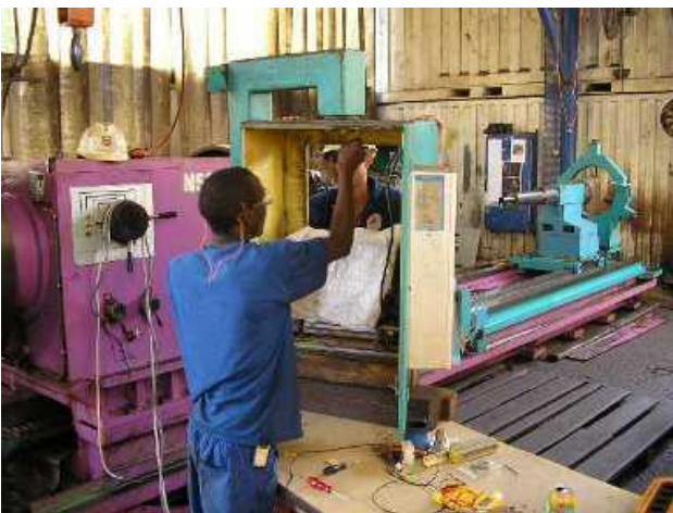
Figure 6: Dismantling of old CNC
