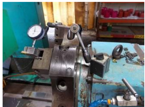
P16: The turret must be without play, otherwise it will vibrate during rotation. This means that the quality requirements are not met.
