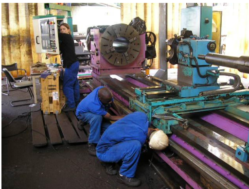
Figure 12: Here, the Z carriage is lifted
