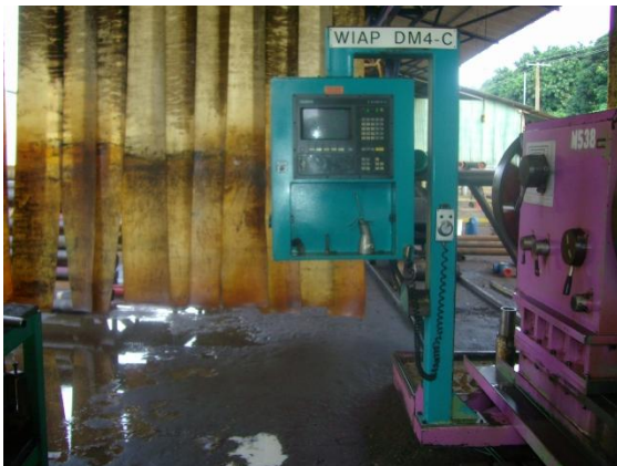
Figure 1: The second modification of the machine. Cultivation remodeling one on Sinumerik 810. Tag 2: Sinumerik 802
