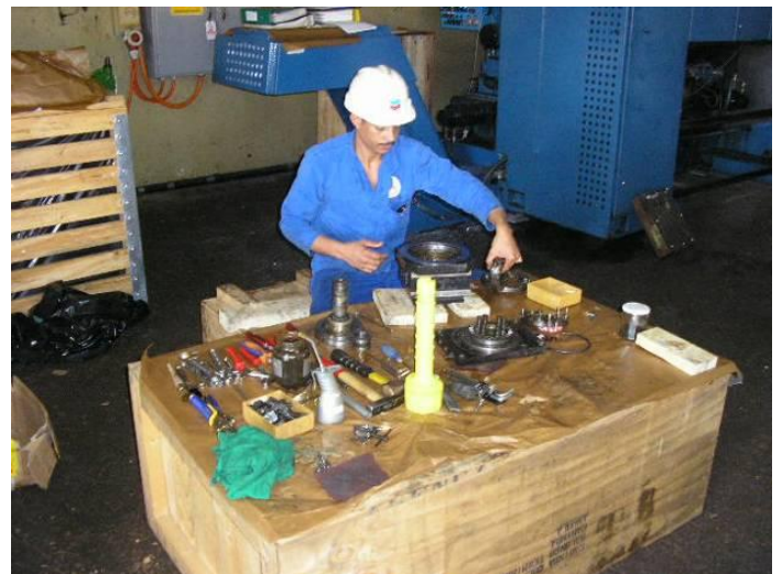
Figure 17: Carlo starts with the assembly. A clean workplace is important that oil paper also.
