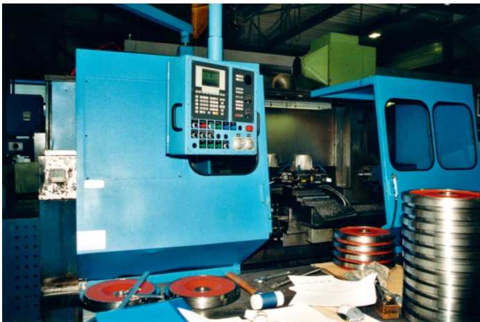
Figure 1: Graziano SAG lathe with a new CNC control
