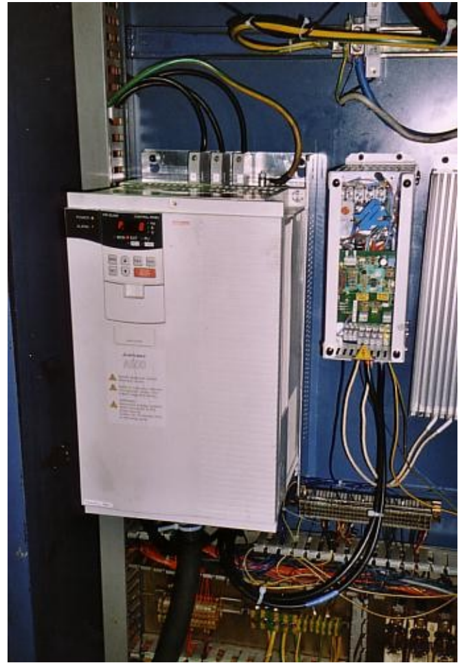
Figure 8: New spindle drive for Graziano CNC lathe.
