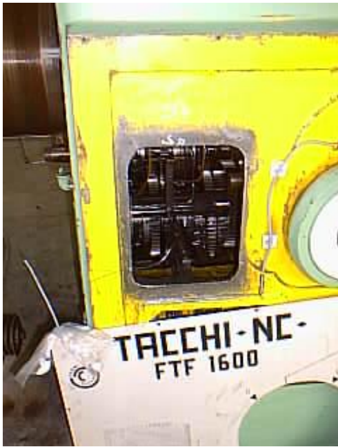
Figure 6: Repair headstock Tacchi
