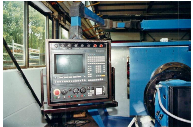
Figure 2: Installation of new CNC with commissioning and training
