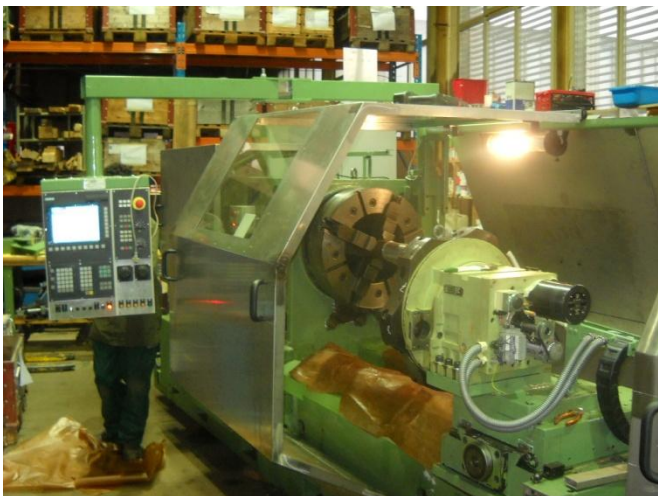
Figure 25: Now is the Olefelddrehmaschine which was converted from a conventional, ready to be delivered. New ball screws. New tool turret; reground bed; reground slide and new with sliding occupied. Newest lubrication system; new spindle drive and much more.
