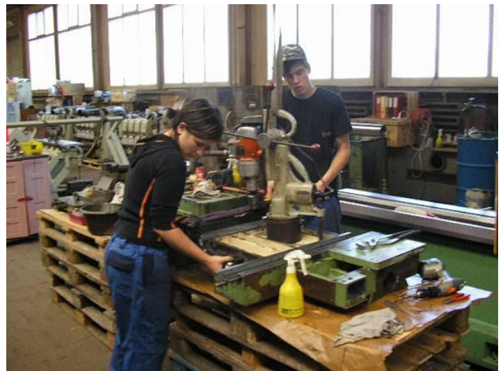
Figure 14: Caroline Widmer drilled new lubrication holes in the sled. WU_260_100
