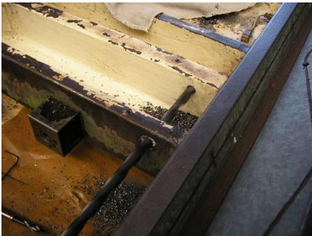
Figure 16: It is so bored that the lubrication lines are mounted on the chip area can. Below is there a cover WU_260_120
