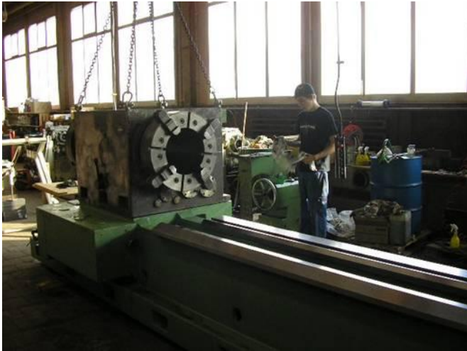
Figure 24: What a Oelfeldspindelstock is difficult. The flight to the Z axis must be perfectly correct. Ideal to 300 mm less than 0.03mm taper that is in radius 0015 and to the right page. As a rule, always forward further away from the lining thinner because the cutting pressure further and further away by the tool from the chuck, expresses more.
