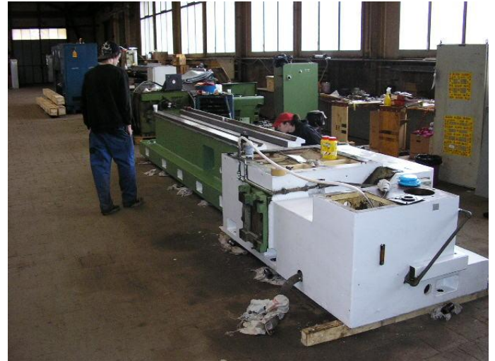
Figure 22: The machine has suffered greatly in Angola, a few meters from the sea. That eats everything, so we bought the best quality color and even matched it with the color supplier before.
