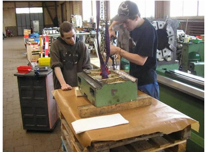
Figure 13: For hours scraping and again put the sled again to the ground pad and abtuchieren. When 10-15 support points on one inch in / 2 is da (25.4 mm / 2), it is ok for old rules. For grinding 25 contact points per / 2 inches are required. WU_260_90
