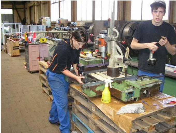
Figure 15: This requires some force. However, there will be many new lubrication holes, as the machines short stroke, investments like these Oelfeldgewinde, often drive only about 150 to 200 mm Dauerwegbereich, has enough lubrication in both axes X and Z. We have min. 3 made x more lubrication points , WU_260_110
