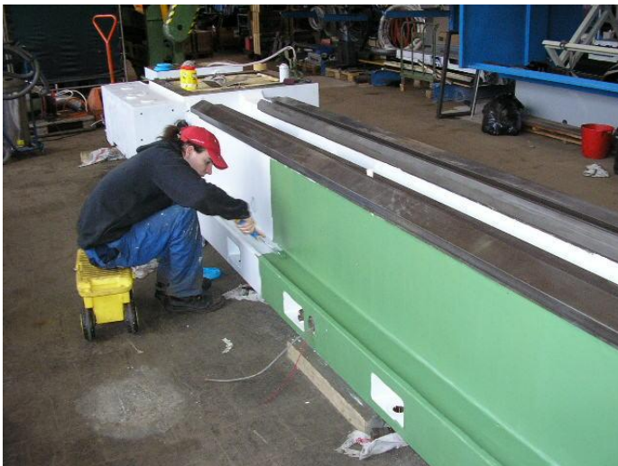
Figure 20: To bring a heavy machine bed in a painting is complex and complicated, while a machine back construction. But it takes 100% discipline. clean clean, good 2 K color which is solvent and emulsion-resistant from the primer. And a good quality assurance. Everyone has to controlling the other, that is not sloppy.
