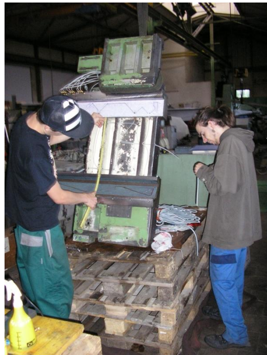
Figure 18: The right sliding layer is the heart of the work. The WIAP has virtually worked with all and utilize the respective necessities. Especially that the stick-slip effect = Haftgleiteffekt, not a negative effect on the precision of the machine tool.
